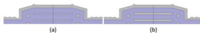
Figure 12. Cold plate designs used for feasibility demonstration of the AM fabrication and experimental characterization capabilities: (a) Model 1: five straight channels with 0.8 mm fin width, and (b) Model 2: five straight channels with 1.6 mm fin width.
