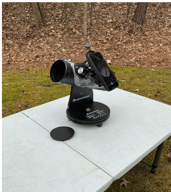
Figure 3. The telescope setup consists of the Celestron FirstScope, an iPhone 15 Pro, a Celestron phone mount, and a folding table.
