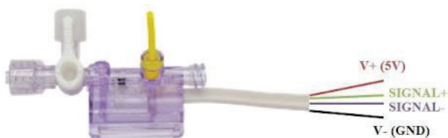
Figure 4. Pin map for Edwards-Pressure Transducer.
