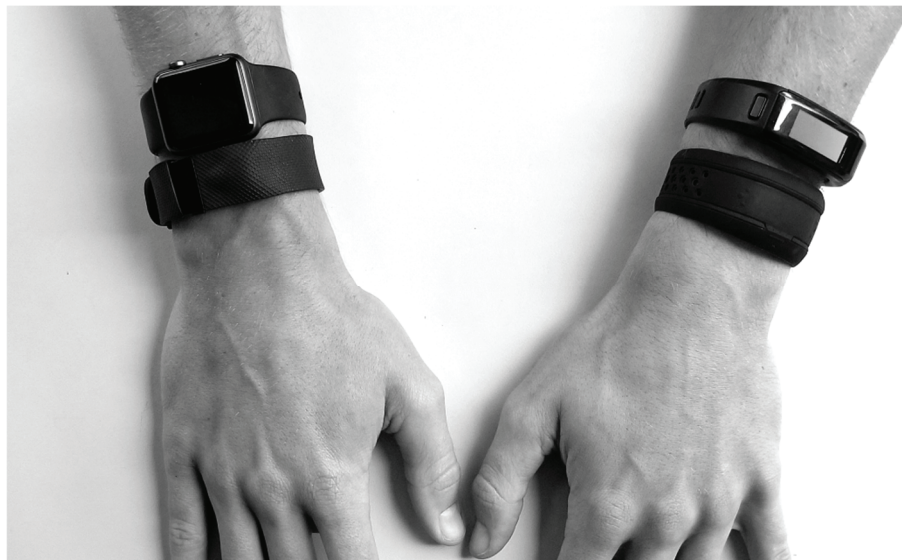
Figure 1. Device Placement. Right arm (Fitbit closer to hand, Apple Watch). Left arm (Mio closer to hand, Garmin).
