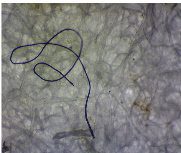
Figure 4. A blue microfiber under a dissecting microscope.
