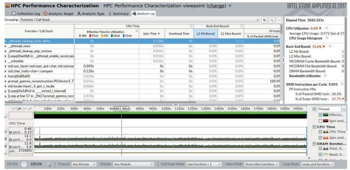
Figure 12. VTune Performance Characterization for the Modified MPI algorithm with 4 processes per node.
