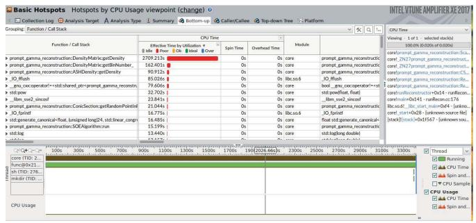
Figure 13. VTune Hotspots Analysis for the Modified MPI algorithm with 4 processes per node.
