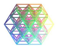
**Figure 4.** A subset of the octet truss. There are only four angles that will be formed by any two edges in this figure: 60°, 90°, 120°, and 180°.
