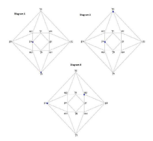
**Figure 10.** in Diagram 1, arms  $\beta_1$  and  $\gamma_3$  are removed from the Schelgal diagram. In Diagram 2, arms  $\beta_4$  and  $\gamma_2$  are removed. Diagram 3 depicts a tile comprised of arms  $\alpha_1$  and  $\beta_3$  which can rotate to fit either Diagram 1 and 2. This occurs because there is an angle of  $2\pi/3$  between each of these arms.
