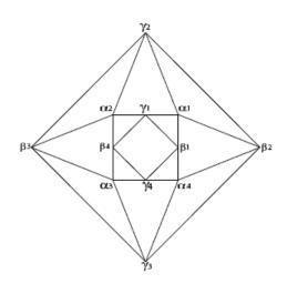
**Figure 8.** This is a schlegel diagram of the cuboctahedron formed by the vertices adjacent to a single vertex in the octet truss and the edges between these vertices. The labels correspond to the endpoints of the arms in Figure 6.
