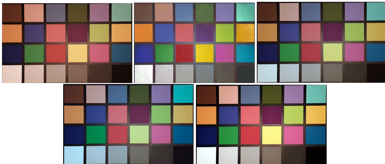
Figure 7. Corrections of an Image from Fig. 2 (left) Using Various Correction Techniques. This figure consists of the original (top left), multi-variable fit (top middle), manual white balance (top right), automatic white balance (bottom left), and 1% saturation (bottom right) methods. Note that, due to its use of the actual chart RGB values, the multi-variable fit image is the most accurate and can, therefore, be used when visually comparing the images for accuracy.
