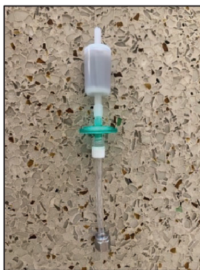
Figure 1A. Ozone scrubber.
