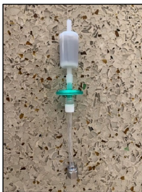
Figure 1A. Ozone scrubber.
