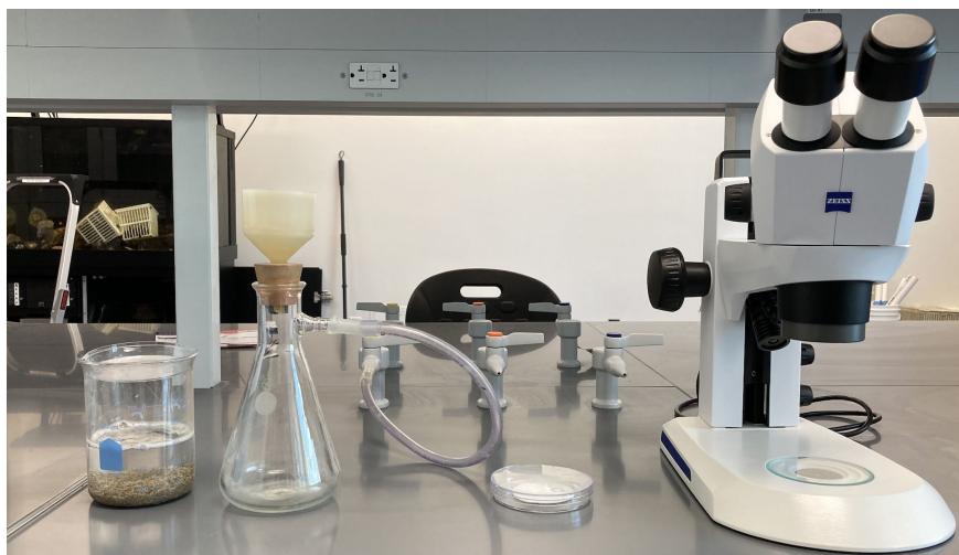
Figure 3. The process by which microfibers were stratified out from sediment, filtered, and observed.
